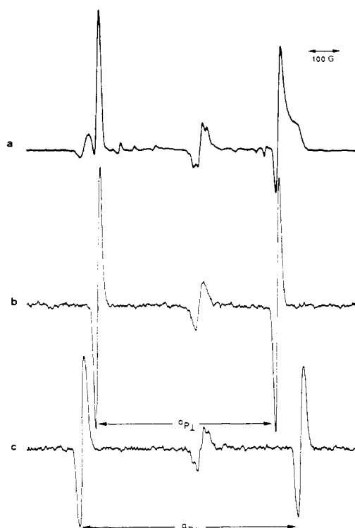
Figure 2. ESR spectra of 1a : (a) powder spectrum, (b) single-crystal ESR spectrum, H_0 parallel to the c axis, (c) single-crystal ESR spectrum, H_0 parallel to the b axis.
